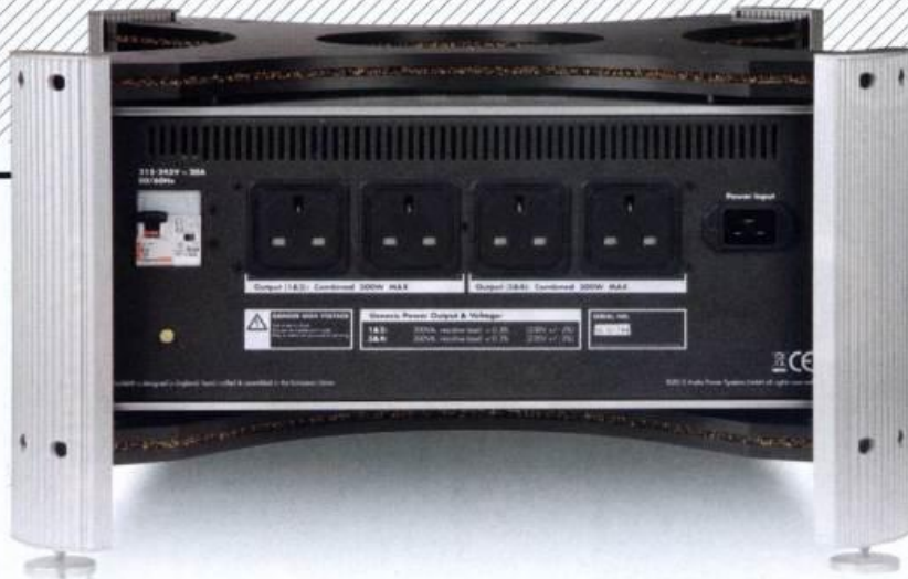
ABOVE: Four output sockets are provided, divided into two pairs which can be separately energised or disabled. Each pair is able to deliver a maximum of 300VA, which is sufficient for front-end components only – not power amplifiers
