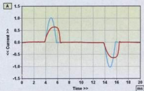
ABOVE: Distorted mains (charging) current waveform (red) versus significantly more linear waveform delivered by the IsoTek EVO3 Genesis (blue)
