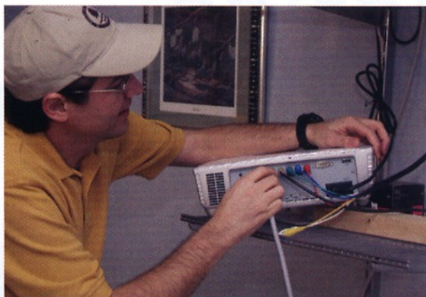
A The Optoma's clean, uncluttered back panel still offers connections aplenty, including HDMI and DVI inputs.
