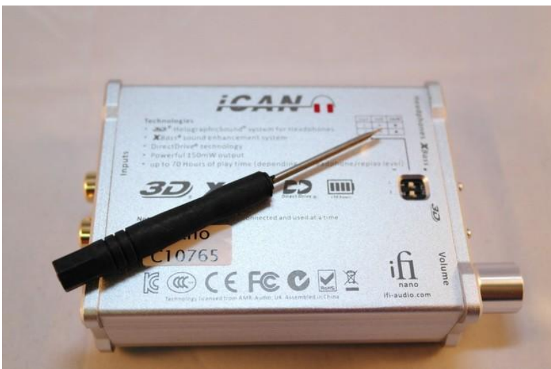
The gain switch on the bottom of nano iCAN
