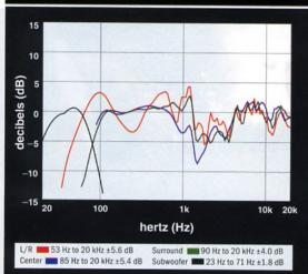
The Vienna Acoustics' unusual driver arrangements deliver frequency response that varies widely by horizontal angle, meaning that listeners tend to get different sound based on position. The REL sub had uniform output from 32 to 62 Hz, averaging 102 dB SPL; max output was 107 dB at 62 Hz with 10% distortion. But it lacks dynamic capability. delivering just 84 dB at 25 Hz with more than 20% distortion. - Tom Nousaine
