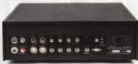
The Vivaldi DAC's rear panel offers every digital input other than Ethernet.
